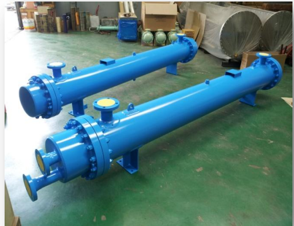
Lube Oil Cooler (Camermon)
