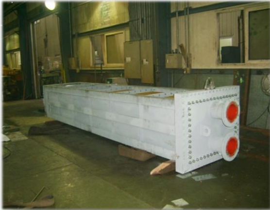
Gas Cooler (Hyundai Steel)
