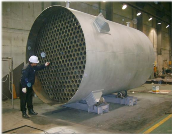
Water Cooler (POSCO)
