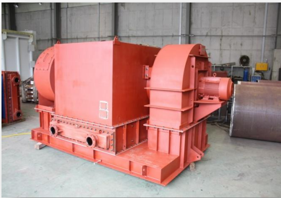
Motor Cooling Unit (TMEIC)
