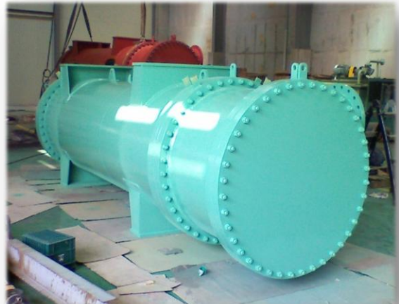
Water Cooler (POSCO)
