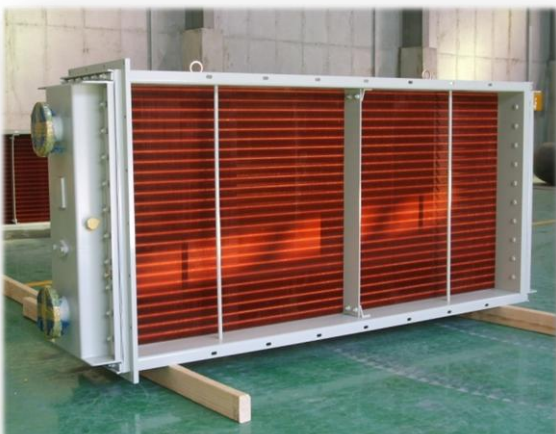
Air Cooler (Sewoong Plant)
