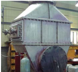
Heat Recovery Unit System
